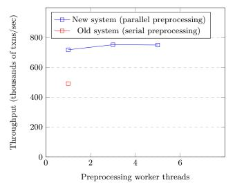
Here we see that the new system even with a single worker thread (effectively performing preprocessing work in serial) offers a near 50% throughput advantage over the old system. Also interesting is the observation that the performance does not significantly improve as more preprocessor worker threads are added to the system.
